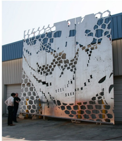
EXTERIOR SURFACE OF WATER JET CUT ALUMINUM PANEL SYSTEM DURING FABRICATION PROCESS BEFORE BEAD BLASTING AND PAINTING
