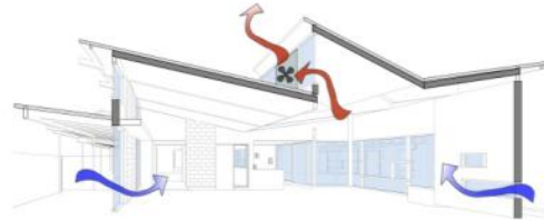
Natural ventilation with fan assistance
