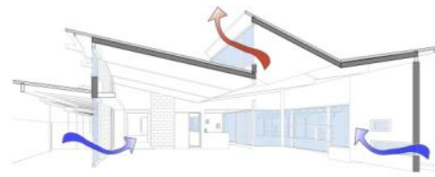
Natural ventilation intake low, exhaust high
