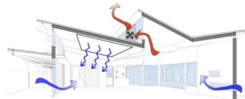
Natural ventilation with fan assistance and radiant cooling
